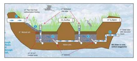
"The gravel wetland does an exceptional job of removing nearly all of the pollutants commonly associated with stormwater treatment
