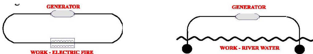
Figure 1 - Simple circuit (left) and electrofishing circuit (right)
