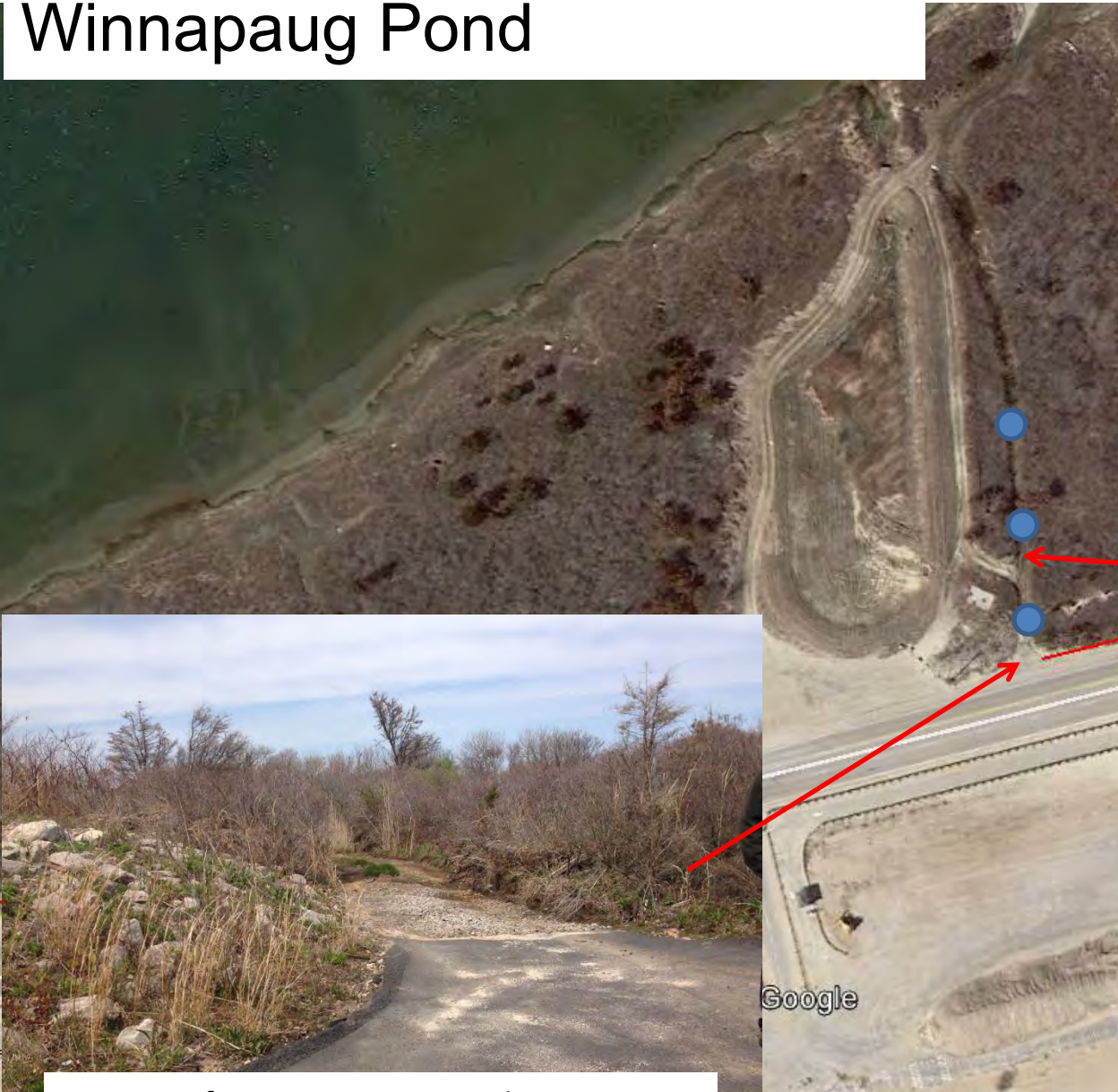
Area of pavement removal to create sediment forebay and filter strip
